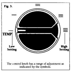
The temperature control knob gives you control over the water temperature in your central heating radiators, and you can adjust it to any position within the indicated range (as shown in Fig. 3.).
