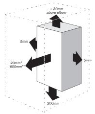
\*600mm service clearance required to a fixed surface (\*\*20mm from removable door or panel)
