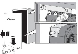
The Flue Thermostat Reset Button (A) and Heating Thermostat Reset Button (B) are located beneath the boiler control panel.
