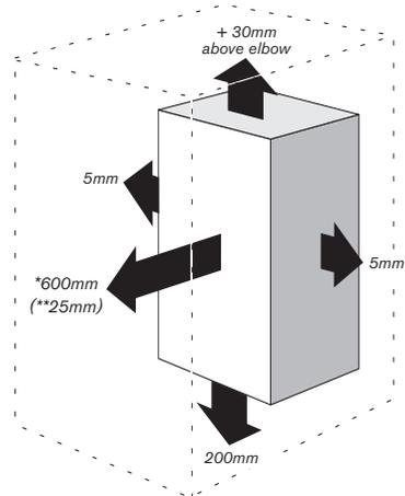
\*600mm service clearance required to a fixed surface
