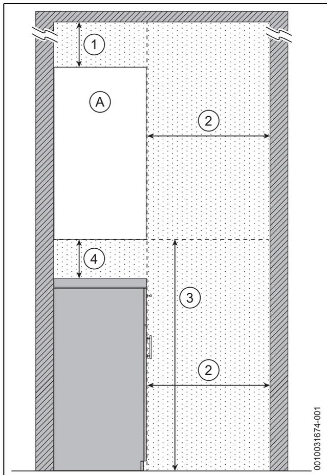
Fig. 8 Reduced front maintenance clearances - Side view
