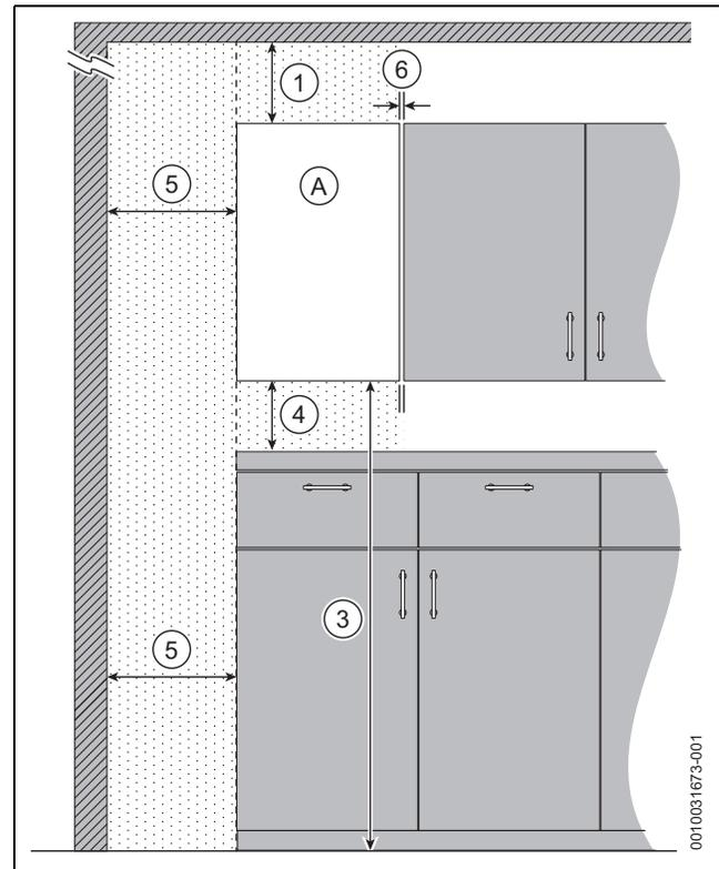
Fig. 9 Reduced front maintenance clearances - Front view
