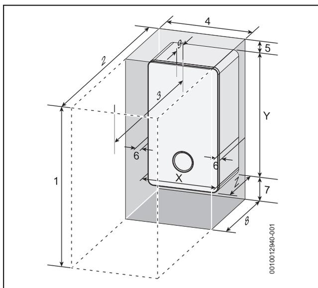
Fig. 7 Appliance minimum clearances
