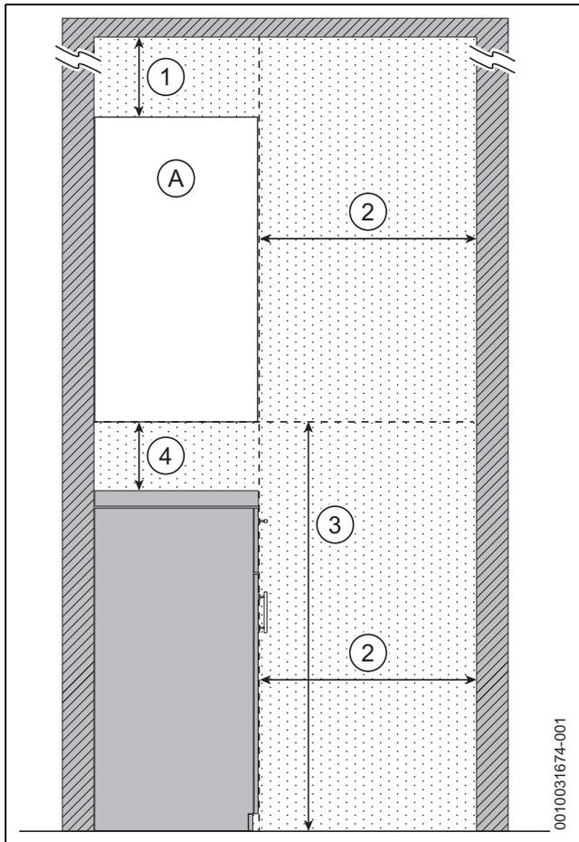
Fig. 11 Reduced front maintenance clearances - Side view
