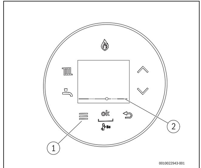
Fig. 2 Pressure indicator for checking the operating pressure
