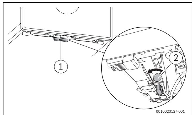
Fig. 6 Locking mechanism
