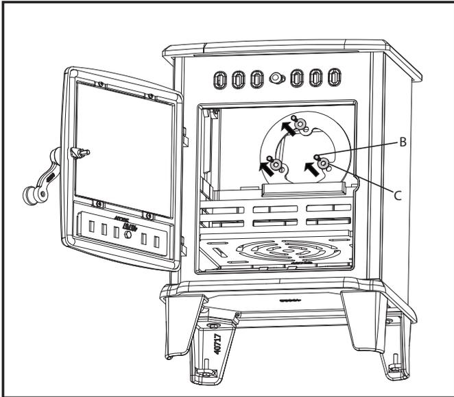
2. Reach in through the front door of the stove and remove the three (B) bolts, and (C) washers, that are holding on the flue collar.
