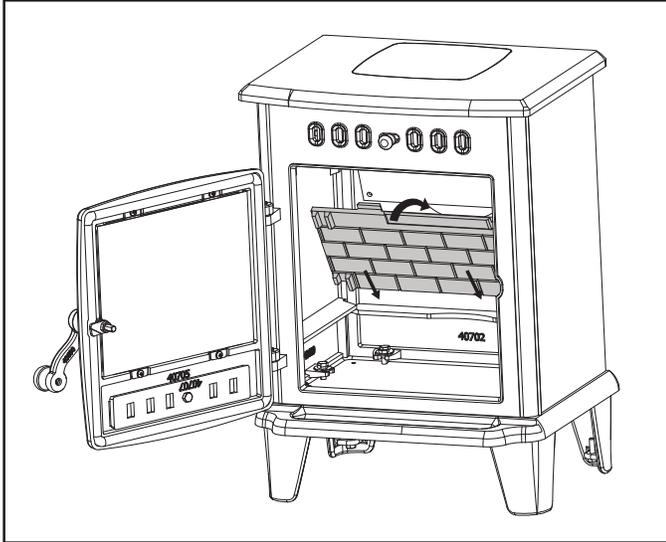
2. Next install the grate. Note that there are two small notches and two large notches. The two large notches must face the front of the stove or the grate will not correctly install.
