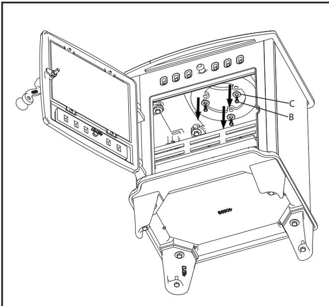
3. Attach the flue collar to the rear of the unit with three (B) bolts and (C) washers.
