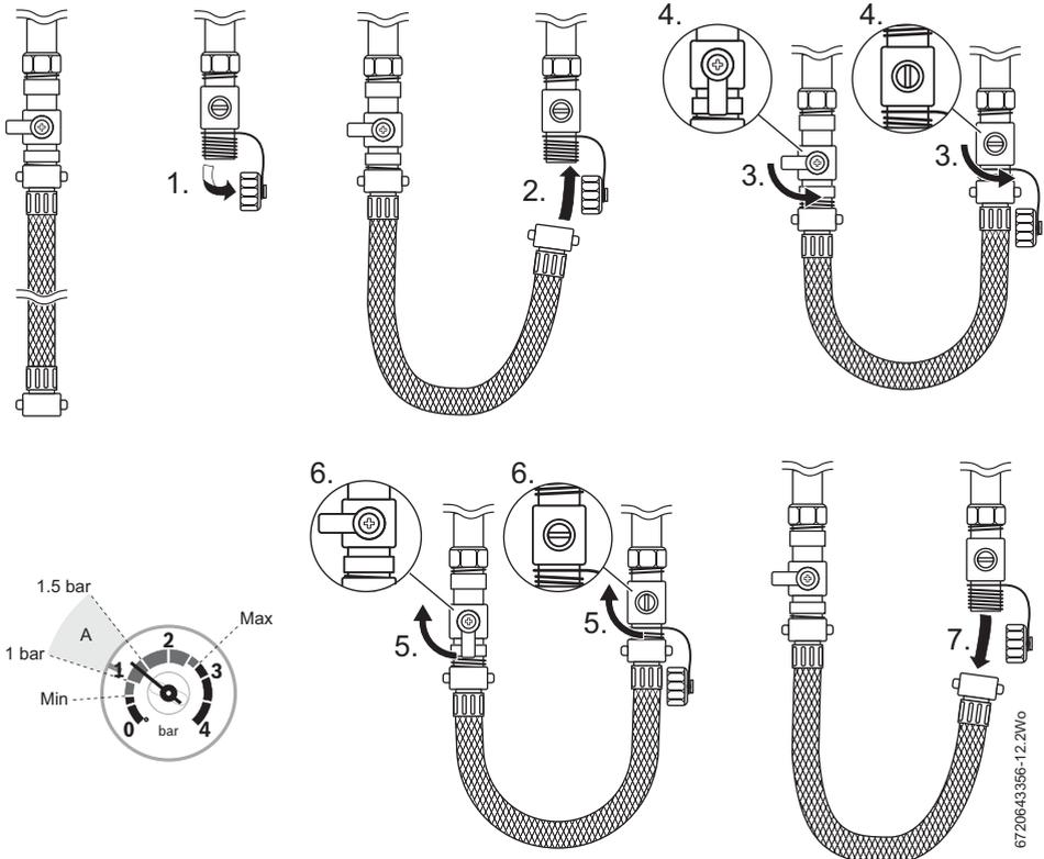
Fig. 10 External filling loop
