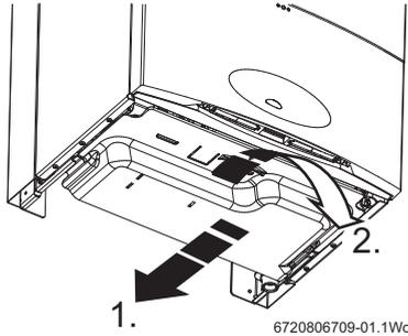
Fig. 6 Remove the bottom panel
