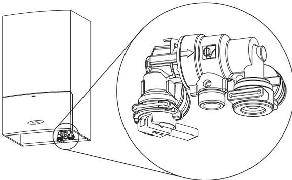
Fig. 7 Integral filling link location
