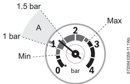
Fig. 6 Optimum pressure when cold (area A)
